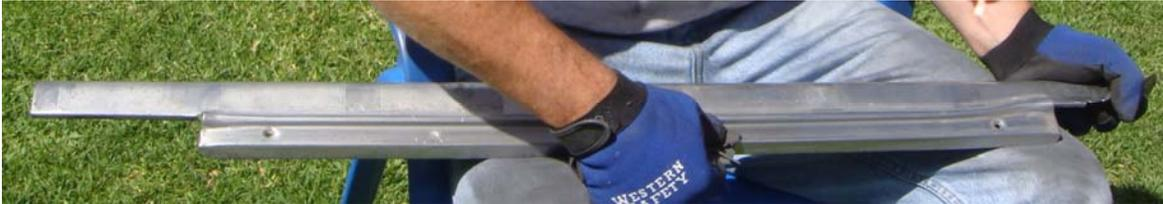
Once everything was sanded and basically polished with 1000 grit paper, I started polishing with an abrasive polishing paste. Since these are long and flimsy, I found it easier to clamp them to the table and use the polishing wheel on my drill.
