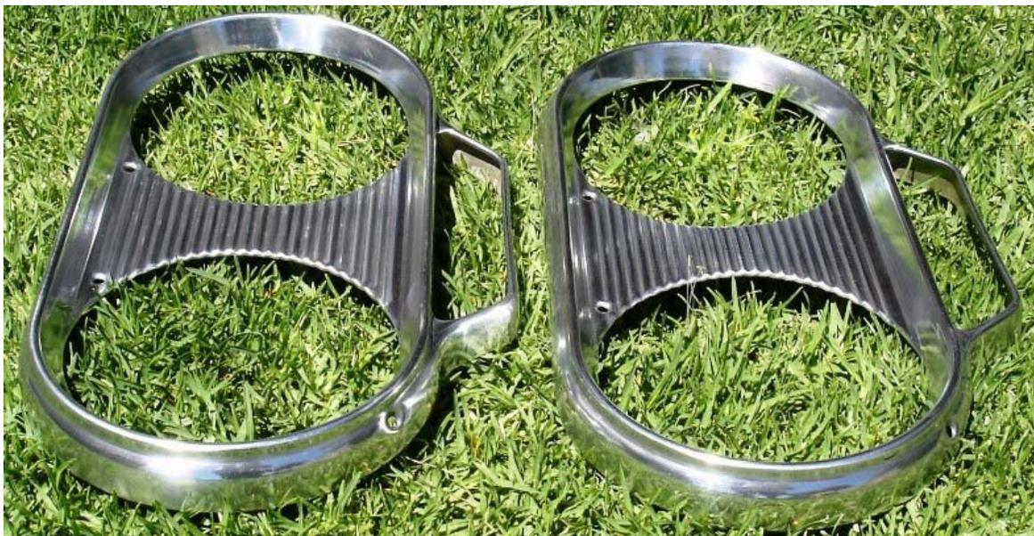
Putting these together with the stainless headlight rims that I straightened and polished, as well as the headlight housings that I sandblasted, patched, and painted, the headlights are ready for assembly on the car.
