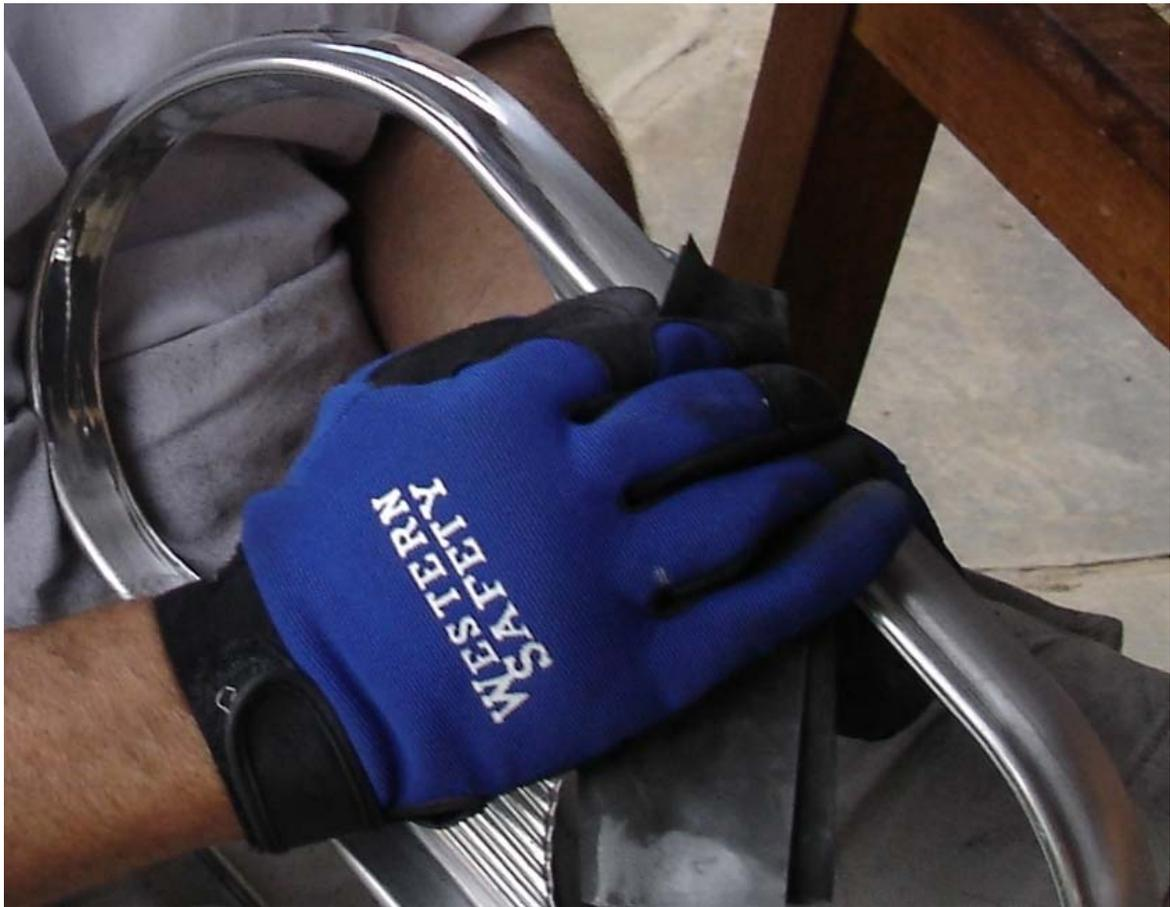
The bezels have small grooves that required the use of a little ice cream spoon on the sandpaper to get into the grooves, followed up by the white polishing stick and a polishing wheel on my mini-grinder.
