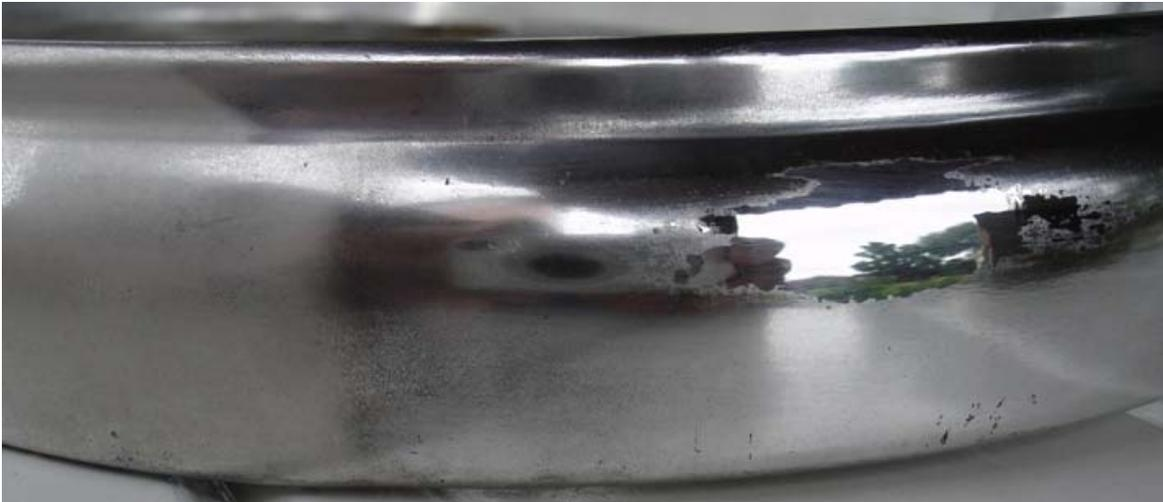
Looking on the internet I found a recommendation to use caustic soda (drain cleaner) to remove the anodizing. This starts bubbling and I used a brush to keep fresh solution where it was needed.
