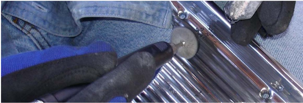
The bezels have a lot of curves, so I combined the polishing wheel on the grinder for the outside and one on my drill for the inside, clamping the bezels to the table.
