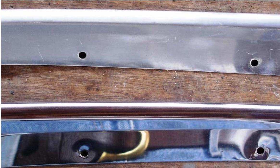
Once all pieces were sanded and polished, I added a little wax and put the pieces aside until the body was repaired and painted. Here is the finished set of belt trim.
