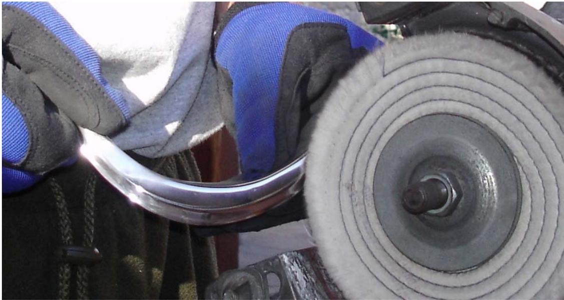
This is a small Craftsman grinder with a polishing wheel. I tried different polishing pastes and compounds, finally realizing that the white polishing stick was the best at taking it to a good shine without caking, followed by a red polishing stick for the mirror finish.
