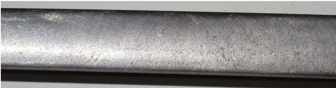
I first tried 150 grit paper, and quickly found that while it took damage off quickly, it left big scratches that were hard to get out. Jumping up to 320 was taking too long to get the deep pitting out, so I settled on a first pass with 220 grit. It might have been better to use water, but I did not have any waterproof gloves. I do recommend gloves, and used the ones you see. These saved a few knuckles on the grinder.
