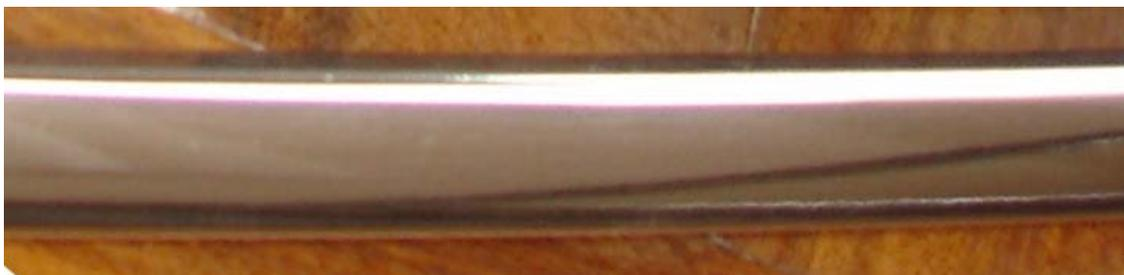
The vertical trim around the roof and windows had a lot less scratches, but the weather had taken its toll. Here is a comparison of two pieces from the roof trim, one before and one after polishing. There were only a few spots on these that required the 220 grit paper. For the most part I started with 360. The reflection is of my jeans and belt buckle.
