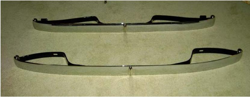
The re-plated bumpers have been attached to the re-painted bumper arms with new stainless capped bolts and are ready to be installed on the car.
