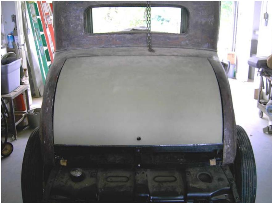
The sheet metal trunk floor pan also fits properly and has been screwed and tacked into place. The similar floor pan that mounts in front of that also fits well, and I will screw it into place soon.
