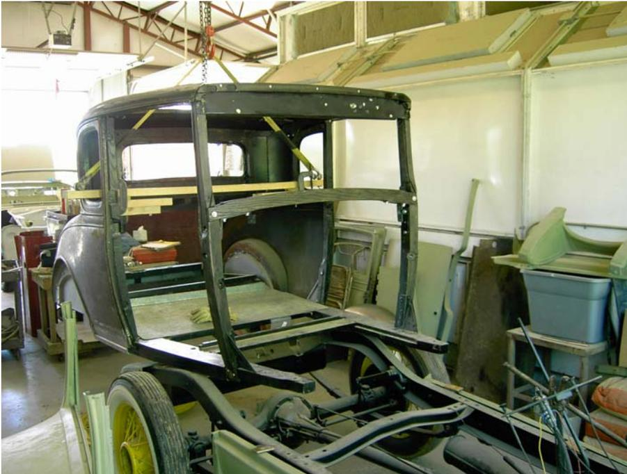
The cowl was then fitted to the body. With the new wood the cowl went into place much more easily and everything lined up properly, so Tommy hammered the sheet metal tabs into place around the wooden door hinge posts.
