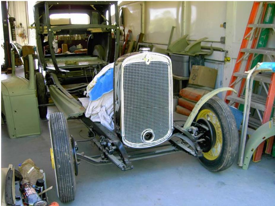
The new wood door hinge posts and roof rails arrived. After checking them for fit, I painted them and installed them on the body, and everything seems to be coming together well.
