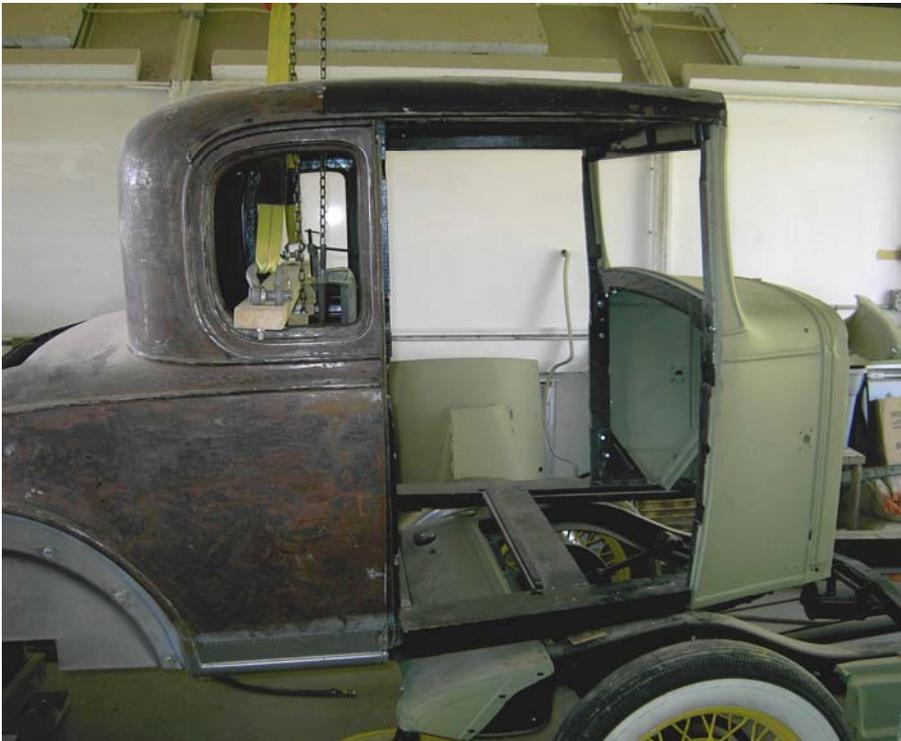
I then put the body back on the chassis and tacked the sheet metal around the opening in the top to the structural wood that supports it. Next I fitted metal trim pieces above the door openings and tacked
